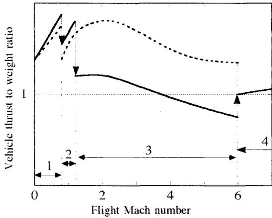
Fig.3 Flight scenario (profile of thrust to weight ratio) for the vehicle powered by KLIN cycle.
