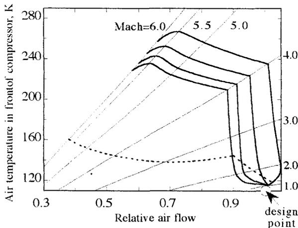
Fig.5 Combined map of the system 'air intake-precooler-compressor'.
