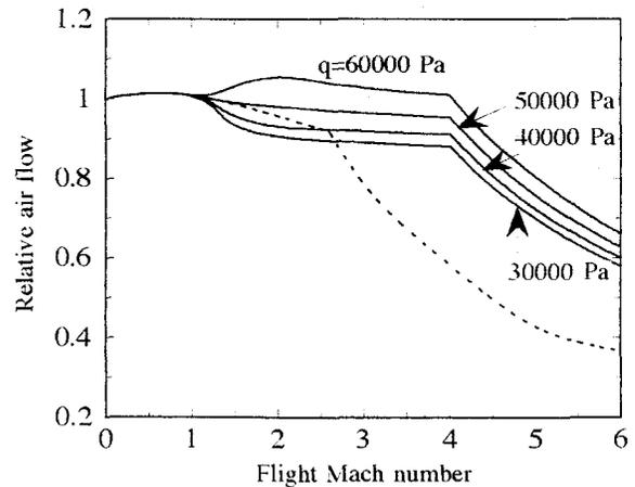
Fig.6 Relative air flow versus flight Mach number for different trajectories.
