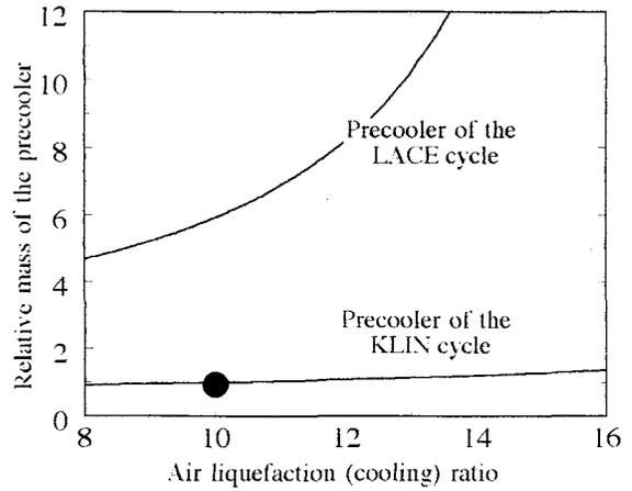
Fig.2 Comparison of the mass of precoolers of the LACE and KLIN cycles evaluated with the same assumptions. Mass of the KLIN cycle pre-cooler at cooling ratio  $K_A=10$  is taken as 100%.
