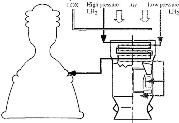
Fig.1 Schematic of DCTJ and LRE thermal integration.
