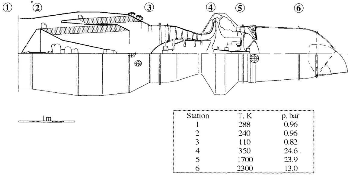
Fig.9 Dimensional configuration of the DCTJ of KLIN cycle.
