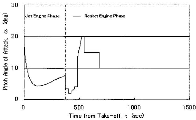
Fig.8a Pitch Angle of Attack
