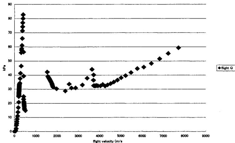
Fig. 11 Trajectory Dynamic Pressure
