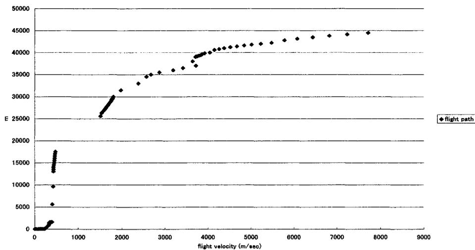
**Fig. 7 Trajectory Altitude vs. Flight Velocity**
