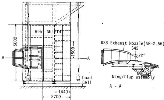
Fig. 3 Geometry of engine-wing/flap assembly.
