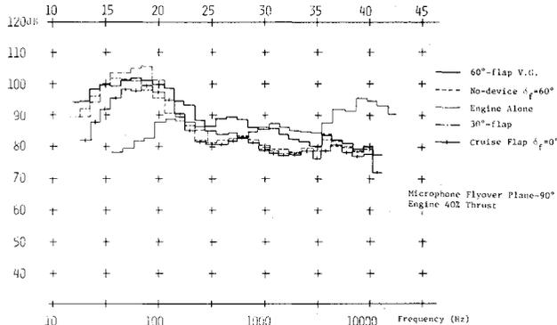
Fig. 4 One-third octave band spectra at flyover - 90 deg direction.
