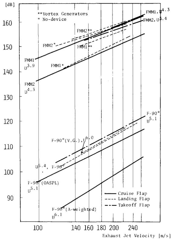
Fig. 7 OASPL dependence on exhaust velocity.
