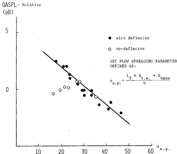
Fig. 14 Noise dependence on  $\alpha_{s.p.}$ .
