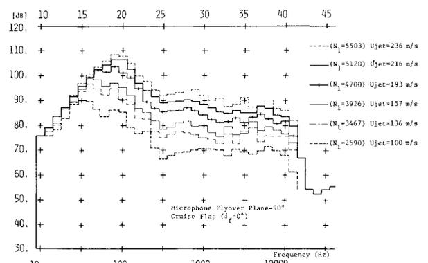
Fig. 6 Effect of exhaust velocity variations on noise spectra.
