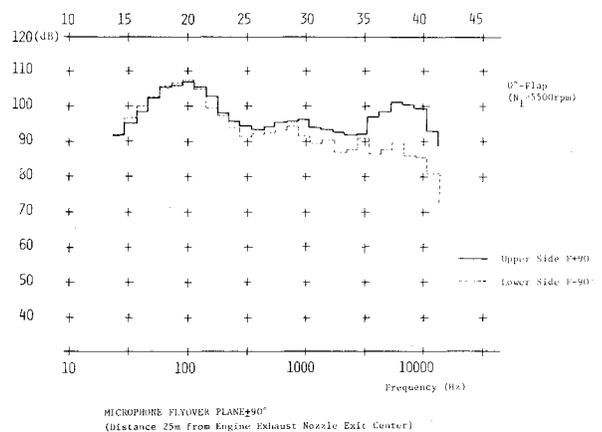
Fig. 11 Comparison of noise spectra at directions below and above the wing.
