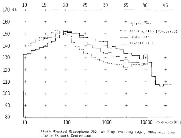
Fig. 8 Fluctuating surface pressure at flap trailing edge.
