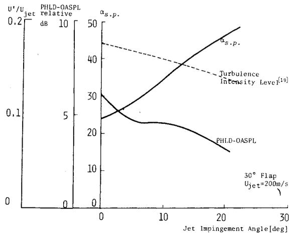
Fig. 15 Effect of jet impingement angle variations on OASPL,  $\alpha_{s.p.}$ , and turbulence intensity level.
