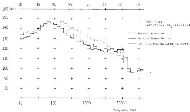
Fig. 13 Effect of vortex generators.
