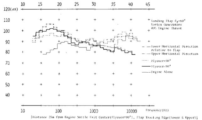
Fig. 5 Comparison of spectra at upper and lower directions for landing flap configuration.
