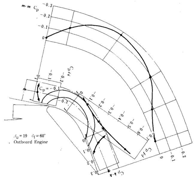
Fig. 4  $C_p$  profiles and contours on side fence surface.
