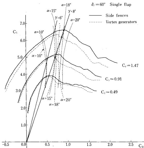
Fig. 10 Lift-drag polars for the landing flap configuration.
