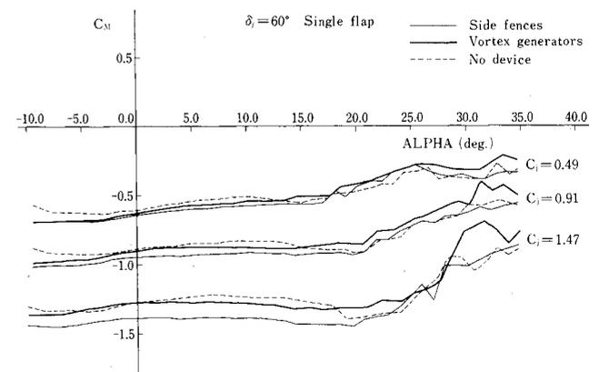
Fig. 9 Effect of side fences on pitching moment coefficient ( $\delta_f = 60$  deg,  $\beta_u = 19$  deg).
