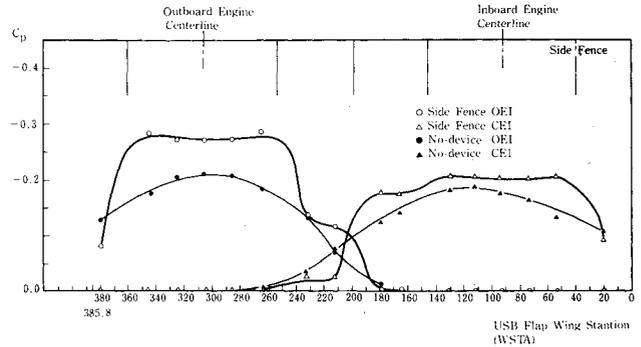
Fig. 3 Spanwise static pressure profiles along midchord line of USB flap ( $\delta_f = 60$  deg,  $\beta_u = 19$  deg).
