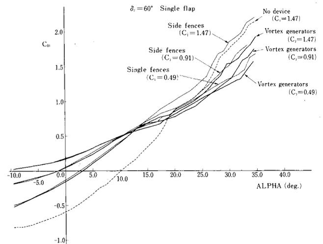
Fig. 8 Effect of side fences on drag characteristics ( $\delta_f = 60$  deg,  $\beta_u = 19$  deg).
