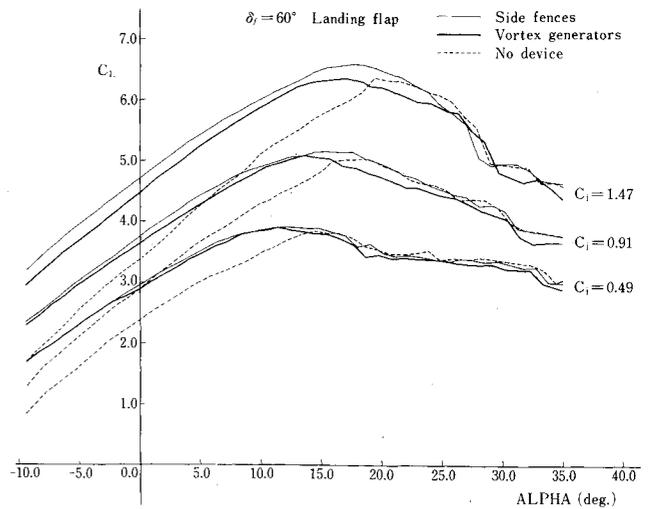
Fig. 7 Effect of side fences on lift characteristics ( $\delta_f = 60$  deg,  $\beta_u = 19$  deg).
