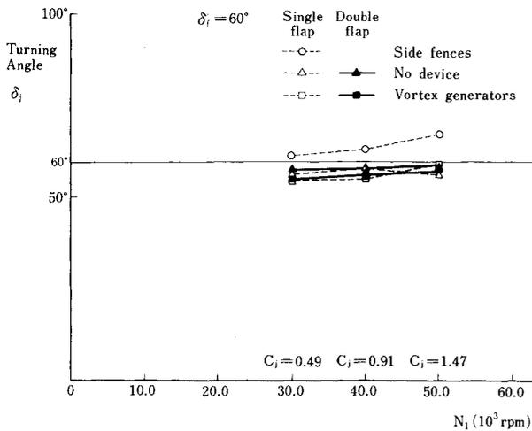
Fig. 5 Effect of side fences on the jet turning performance.
